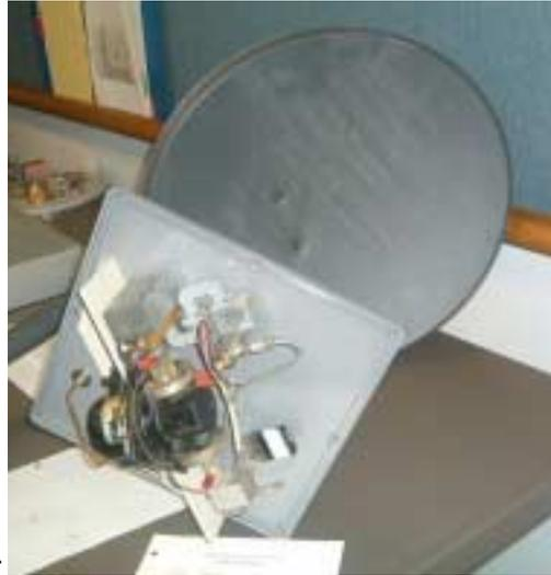
higher bands, with several prodly showing off their 24GHz setups, each unique in their parts and structure. At left is the handiwork of AA3GN, using a small offset feed dish and feed arm as a platform, a weather-proof enclosure for the electronics, and a big waveguide switch as the
