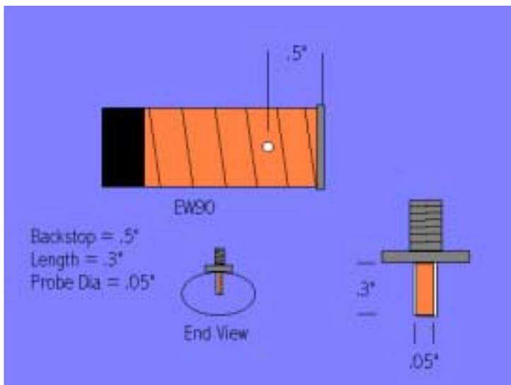
ter of .05" and a conductor length of .3") into a hole drilled .5" from each end of my 95' length of waveguide. I then soldered a brass plate on each end of the waveguide. Proper cleaning and the use of rosin solder flux will assure proper solder flow with minimum heat!
