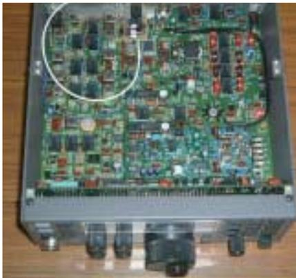
Phil, K3TUF Put together this Elecraft rig and fit a 144-28 DEMI Downconverter Board and a 903 transverter into the cover.
